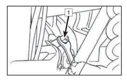
Measure the electrode gap with a thickness gauge, and if necessary, adjust the gap to specification.
